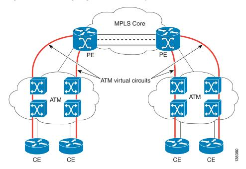
Figure E-7 Configuring AAL5 and Cell Relay over MPLS
